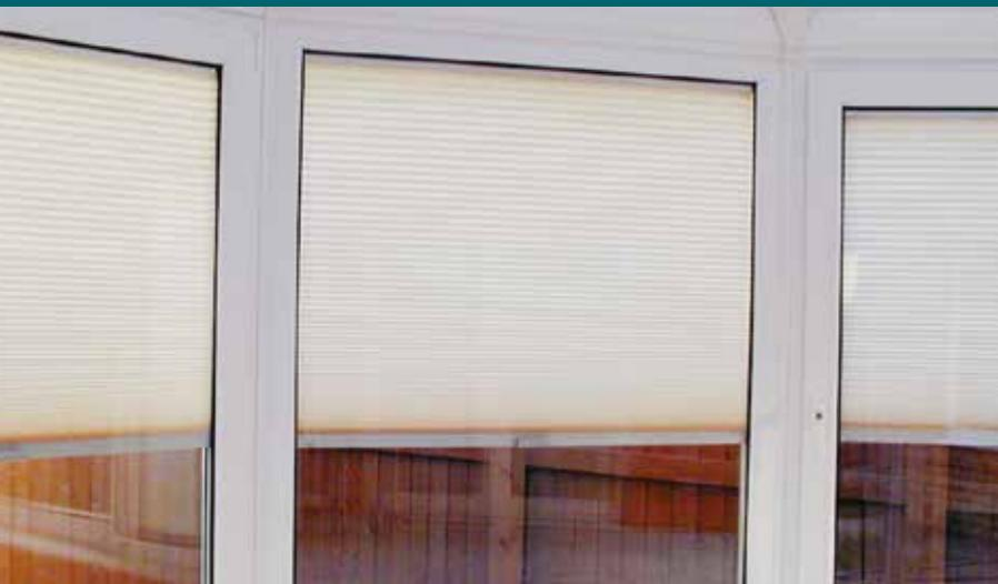
The application of Verosol pleated blind fabrics, coated with an aluminium layer on one side, reduces solar heat gain and improves the U-value, whilst regulating the light passing through. Light transfer down the blind edge is eliminated by the use of special "L" shaped-side guides.
